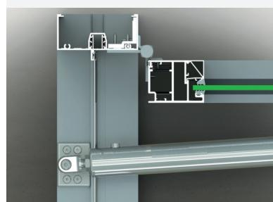
Hinges are secured to Heavy Duty backing plates to ensure the fixings longevity and safety.
